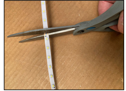
Cut the LED lights to length.
